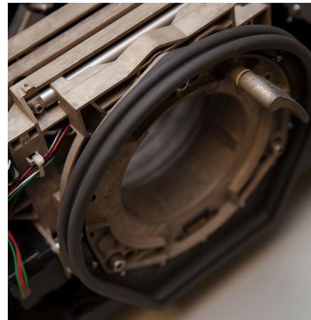
Lens mount boot with rubber-like properties
