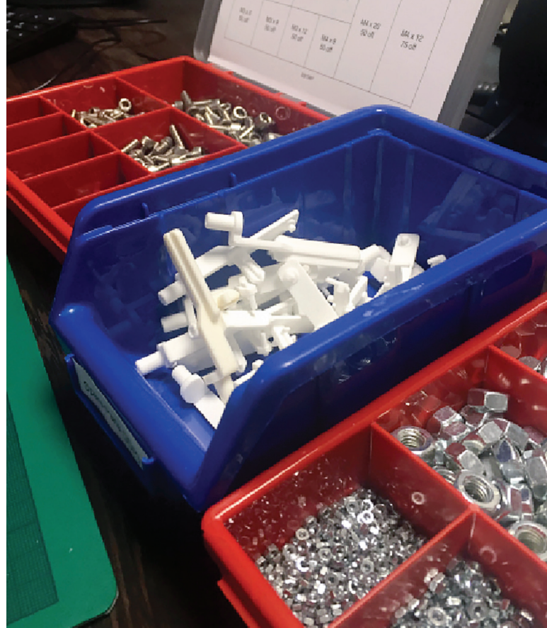
Selective Laser Sintered nylon spare parts.
