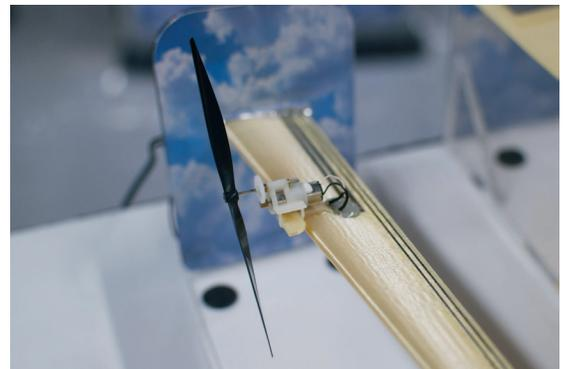
Aurora made this wing entirely of 3D printed components and 3D printed electronics.
