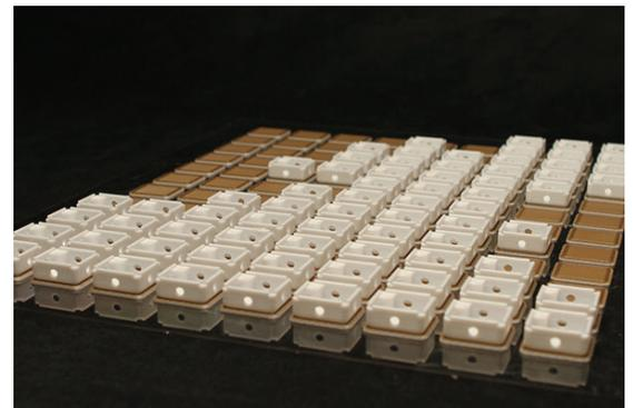
Optimize the orientation and pack of a build for maximum throughput, like these polycarbonate parts.
