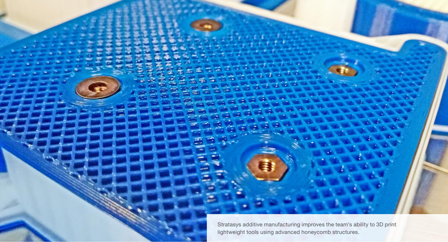
Stratasys additive manufacturing improves the team's ability to 3D print lightweight tools using advanced honeycomb structures.
