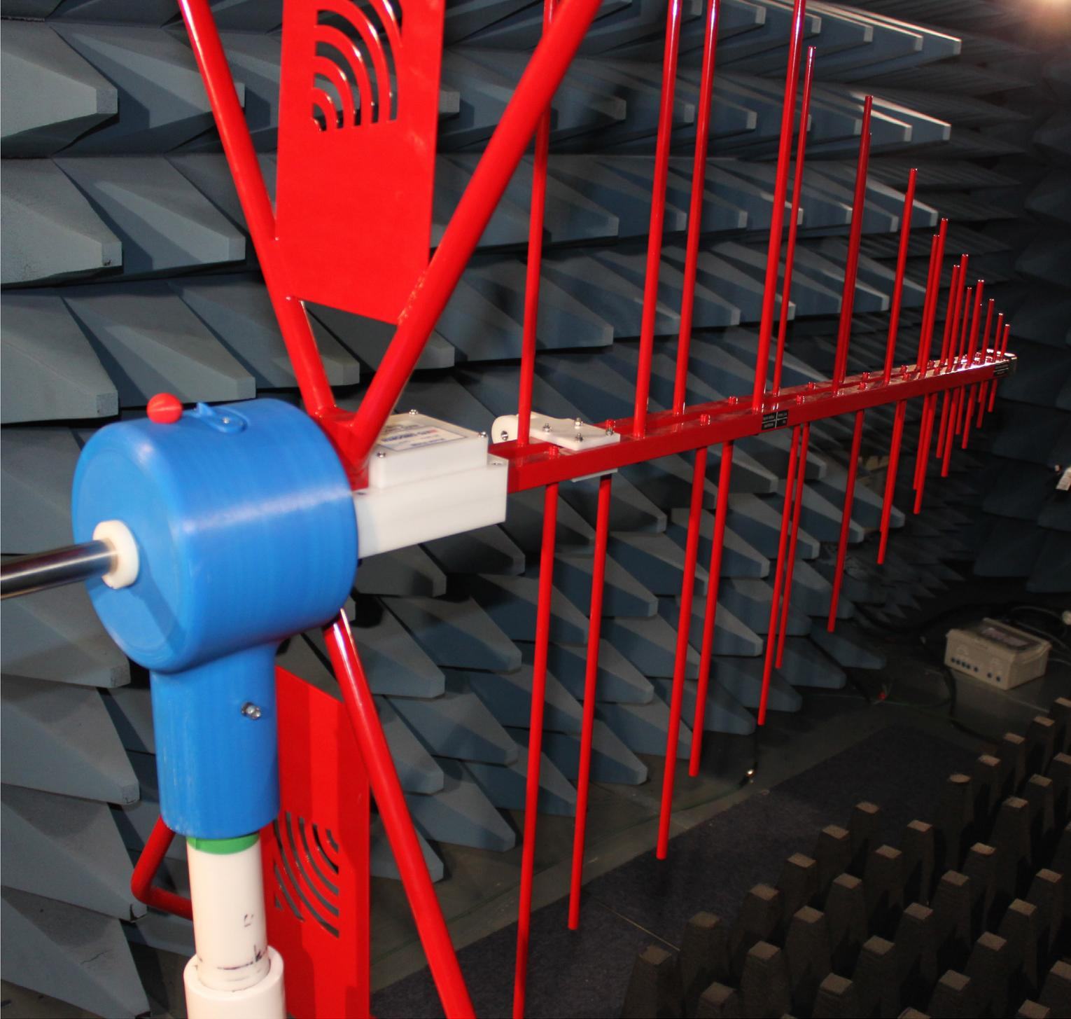
Rotating support for a Bluetooth-testing antenna 3D printed using the Fortus 380mc.
