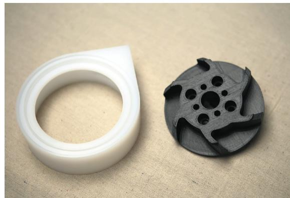
The 3D printed impeller prototype (black) works with its PC mate to push an ice slurry through a chilling system.
