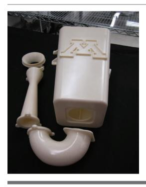
EPOXY SEALED INTAKE VALVE FOR THE UNIVERSITY OF MINN ESOTA COLLEGE OF SCIENCE & ENGIN EERING'S FORMULA SAE VEHICLE
