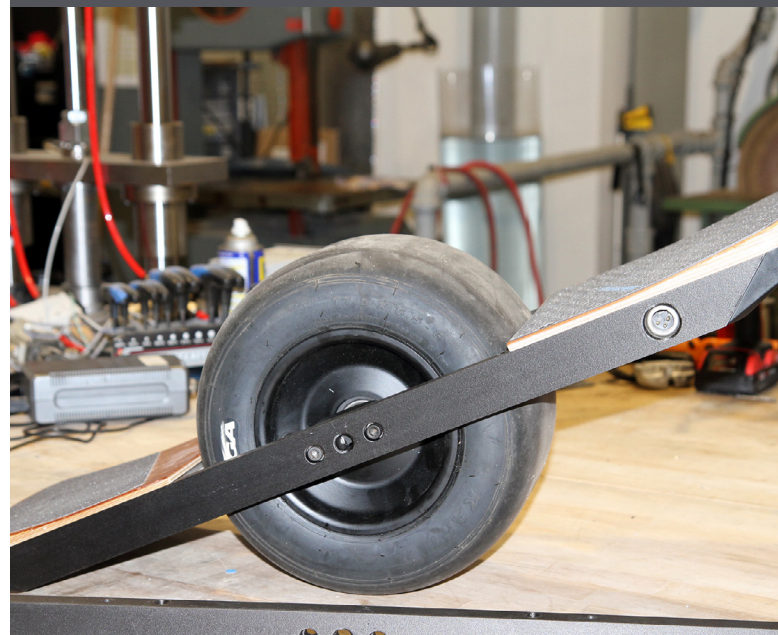
A OneWheel board with carbon fiber nylon (FDM Nylon 12CF) side rails.
