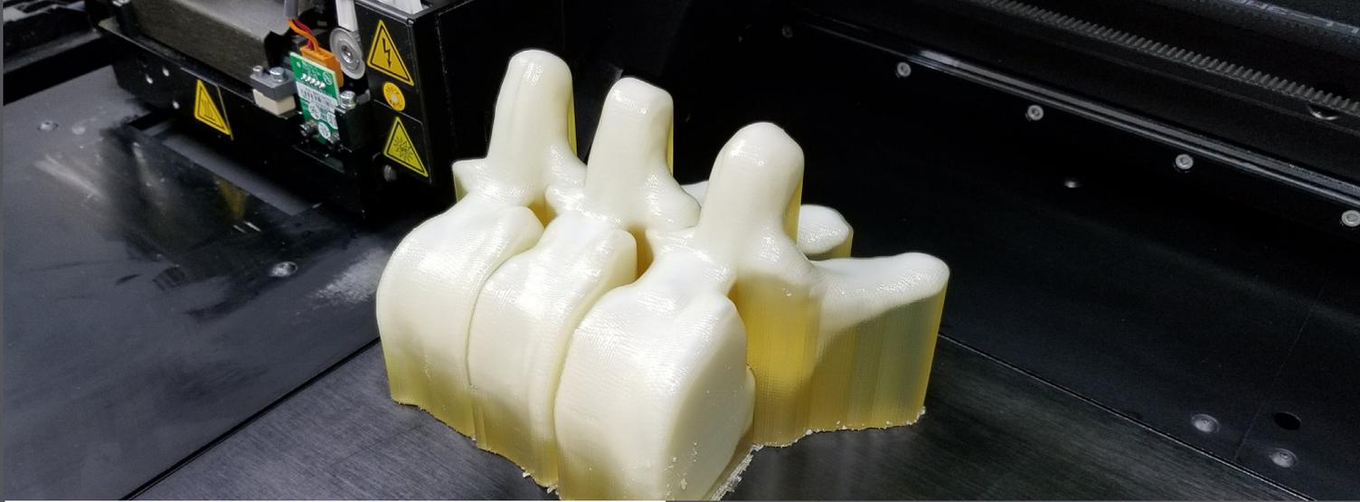
Vertebrae models used for medical device testing, printed on the J750.
