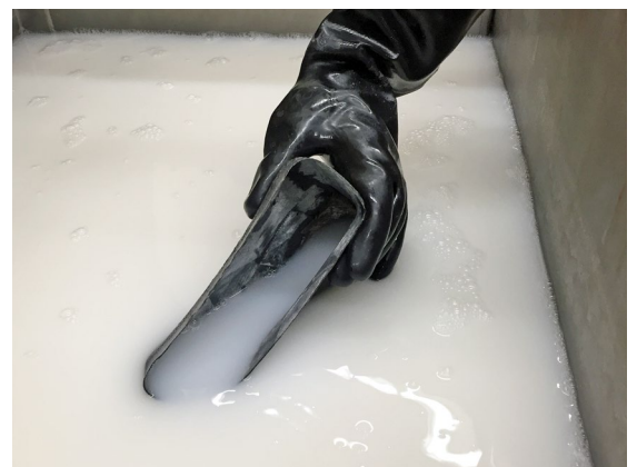
The mandrel used to form this composite brake duct has been washed out, leaving the resultant hollow part.
