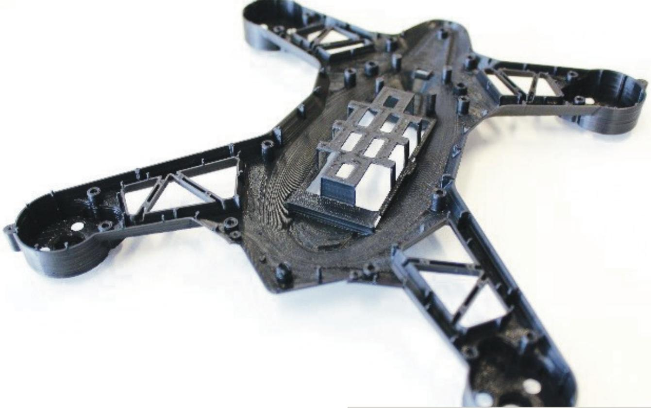
Toy State design team 3D printed frame of a drone with high precision and strength using PC- ABS material.
