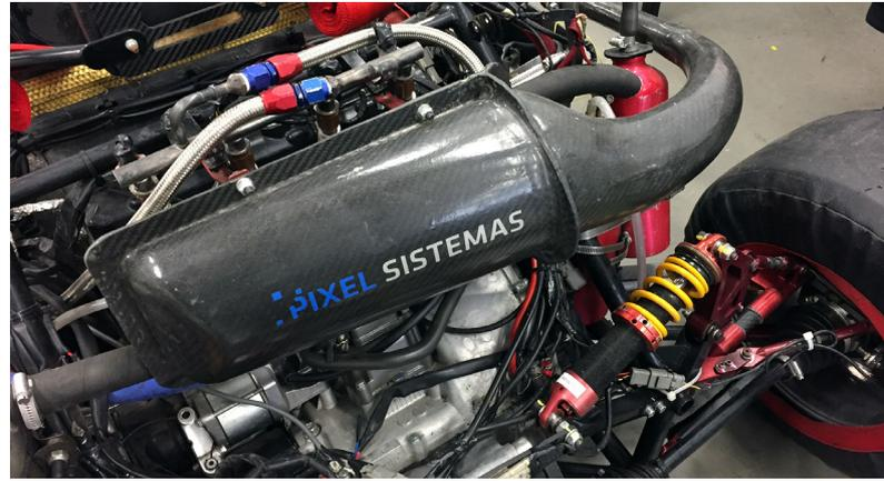
The final carbon fiber intake manifold employs a smooth surface finish for increased airflow and improved track performance.
