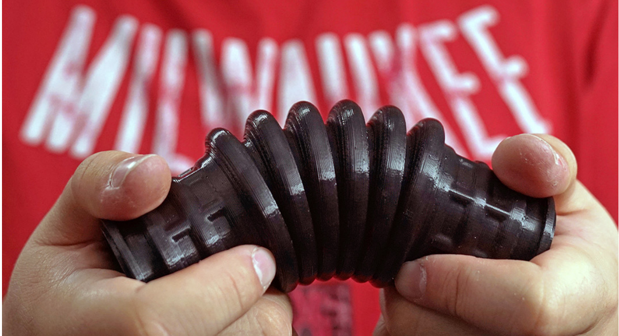
An air intake hose printed in flexible FDM TPU 92A elastomer material.
