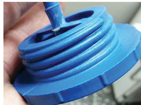
Injection molded screw cap created with a PolyJet mold.
