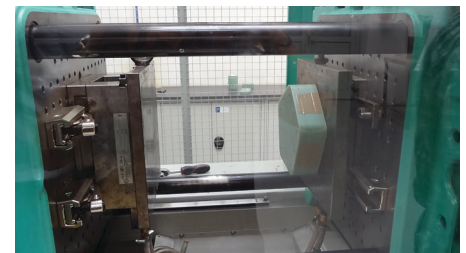
Figure 12: Printed mold for manual ejection.
