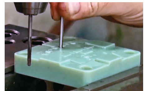
Figure 24: Verifying a snug fit after reaming.
