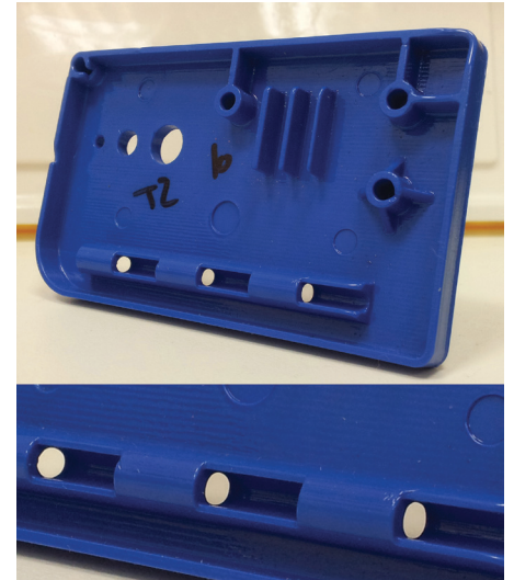
Figure 4: Shut-off for this hinge required no mold modification.
