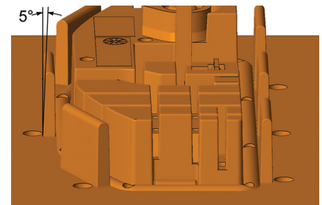
Figure 2: Increase draft angle to ease ejection. Five degrees is recommended.
