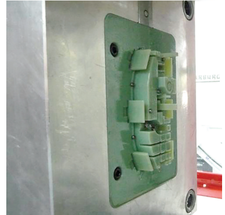
Figure 29: MUD base with the PolyJet core.
