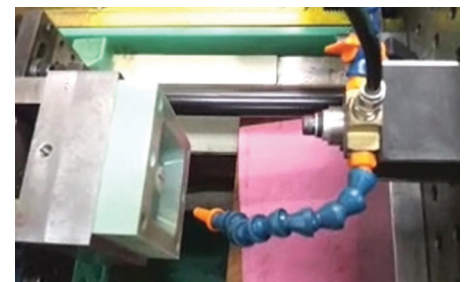
Figure 33: Cooling fixture for blowing air onto the PolyJet mold.
