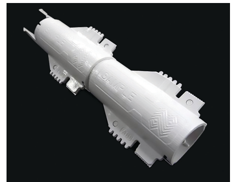
An injected sample part made from ABS material, created by Nypro, to evaluate 3D printed mold performance.
