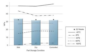
Figure 8a: Tensile strength - 4 weeks, controlled environment, on edge.
