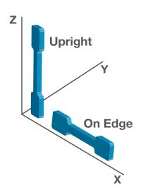
Figure 1: Test sample orientations
