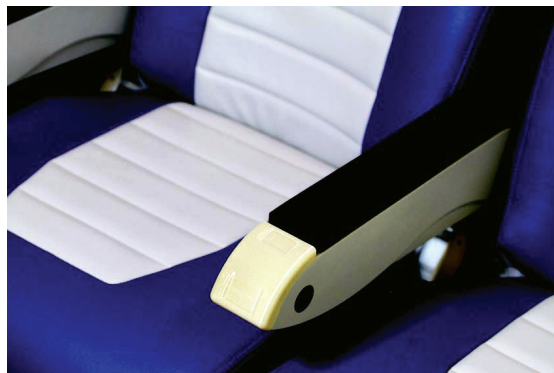
3D printed hand rest for aircraft seats
