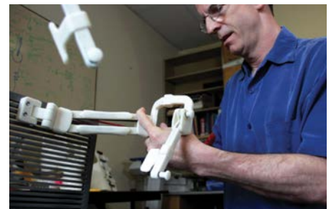
A custom 3D-printed version of the Wilmington Robotic Exoskeleton (WREX) empowers little Emma to use her arms despite arthrogryposis.
