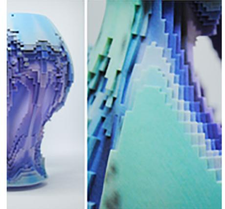
Low resolution 3D printable volumetric texture. Vector-based volumetric textures can be designed and applied to objects allowing them to be fabricated in any resolution with GrabCAD Voxel Print.
