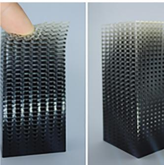
Functionally graded lattice structure with seamless blends of multi-materials.
