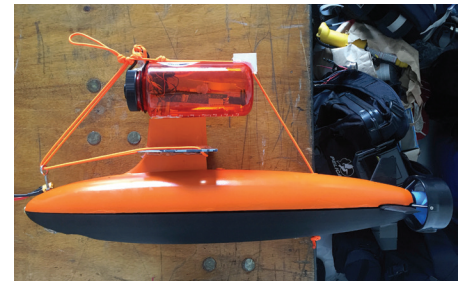
Deployable submarine with camera, encased in 3D printed material
