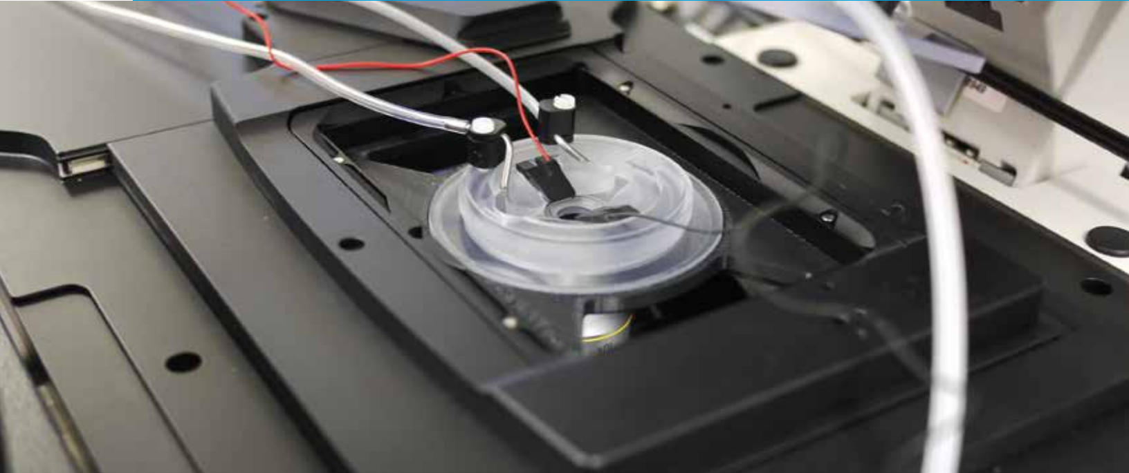
Researchers at the University of Wollongong used FDM and PolyJet 3D printing technologies to build different parts of this watertight and airtight perfusion chamber in a microscope.
