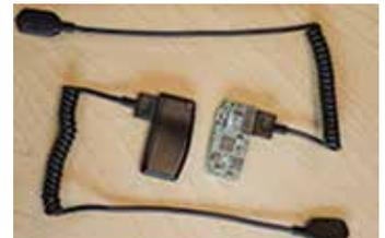
These two accelerometers measure impacts to the head. The one on the left is in a case first tested in a 3D printer and then injection molded. The one on the right shows the circuit board contained in the housing.
