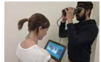
The NeuroTriage system hooked up to a Tablet PC. (top) The tablet controls the cameras and provides the trainers with the results of the test. A student using the NeuroTriage binoculars (bottom)
