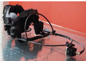
Motion capture devices mounted on helmets, like this one by MOCAP Design, produce high-quality facial movements for the entertainment industry.
