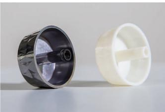
3D printed replacement production part for a crane fan blade.
