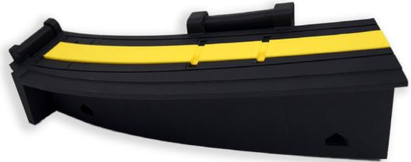
Stratasys FDM additive manufacturing has benefited the Elkamet production floor, shortening lead times of tools, such as gauges, by up to 75%.
