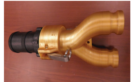
The new design 3D printed in ULTEM 1010 resin cost only $750 and was produced in one day.
