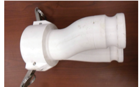
The new Y-shaped design in ABS material wasn't tough enough and cracked during use.
