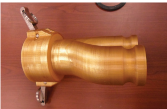
This new Y-shaped design in strong ULTEM 1010 resin has been in production use for eight months without cracking.
