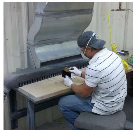
A worker sands ABS-ESD7 next to a dust-collection system while wearing safety glasses, gloves and a respirator.
