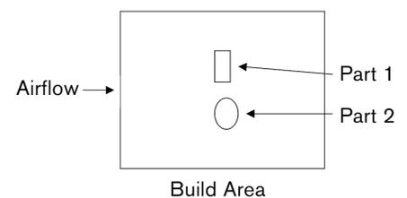
Figure 2: Build area configuration Position parts as close to the center as possible.
