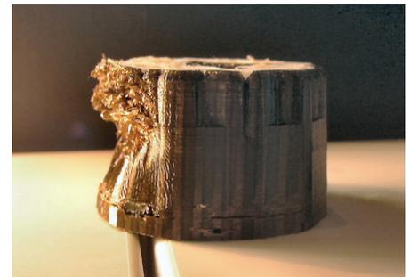
Figure 1: Example of Distorted Part Distorted part due to improper air flow.
