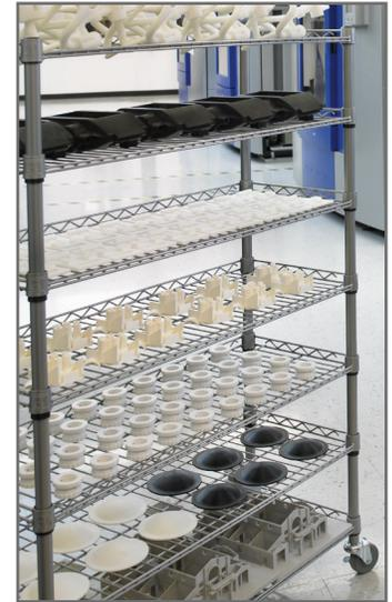
Figure 3: Measure of annual volume - large number of small parts or small number of medium to large parts is ideal for DDM.
