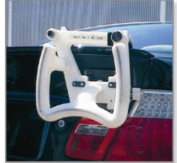
Figure 3: At BMW AG, Regensburg, a FDM-based Fortus system is used to manufacture assembly tools like the one above.
