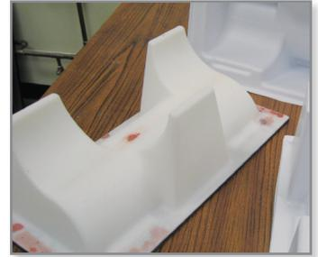
*This FDM thermoforming mold produces drum holders for the manufacturing process.*
