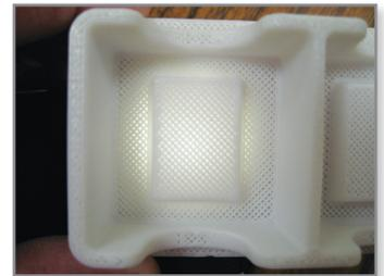
Xerox experimented with various levels of porosity in its thermoforming molds, as shown in this trial fixture.
