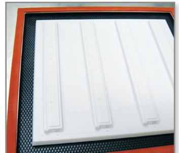
This FDM mold produces printhead covers four at a time.
