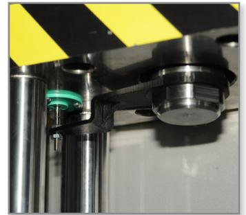
*The ABS drive piece installed in the press system.*
