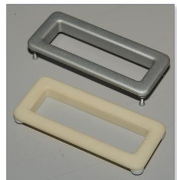
Top: Painted FDM oil level indicator frame. Bottom: FDM oil level indicator before painting.
