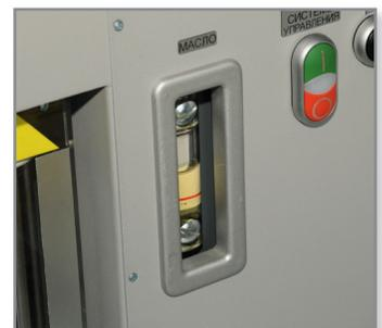
The frame to house the oil level indicator on the hydraulic laboratory press was produced with ABS plastic on a Fortus machine.
