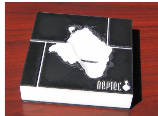
"The Dimension 3D model of the damage to the heat-resistant tiles assisted NASA mission managers in gaining an appreciation as to the extent of the damage. Although the gouge was deep, mission managers believed it posed no risk to the space shuttle's re-entry into the Earth's atmosphere.
