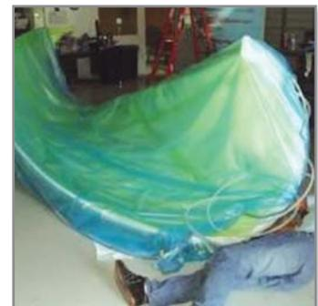
After the skin is laid up onto the FDM core, the composite is placed into a vacuum bag.
