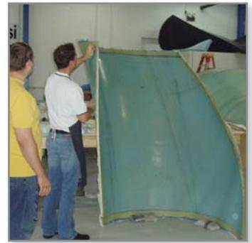
One of several interlocking "sail panels" used to construct a wind turbine blade.
