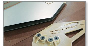
ACS used this FDM fixture as a guide to drill holes in a helicopter fin.
