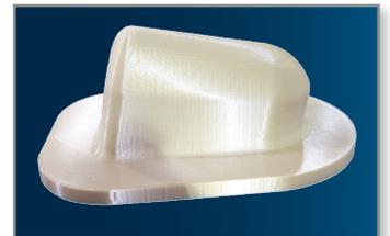
This FDM layup tool produced the aircraft camera fairings above.
