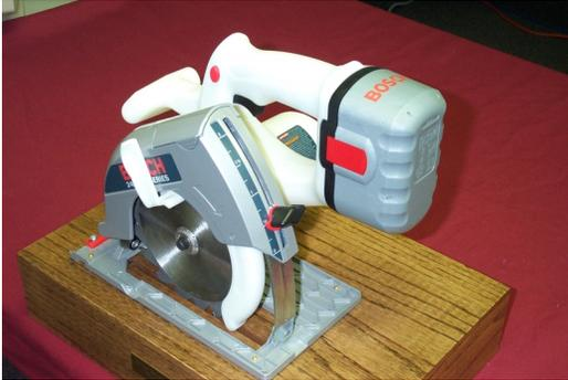
Skil-Bosch uses soluble support material to streamline support removal of prototypes such as this saw.
