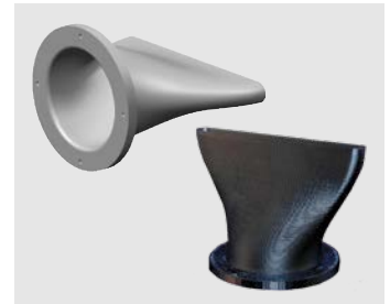
Figure 4: Rear tire blower nozzle for a Joe Gibbs Racing car. CAD model (left), FDM model (right).
