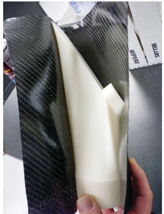
Figure 16: Wrap composite cloth around the core (SR-30 white).
