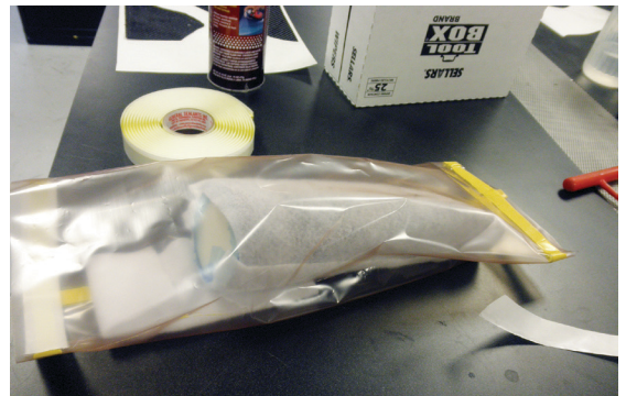
Figure 3: Envelope bagging is one of the consolidation methods compatible with FDM soluble cores.
