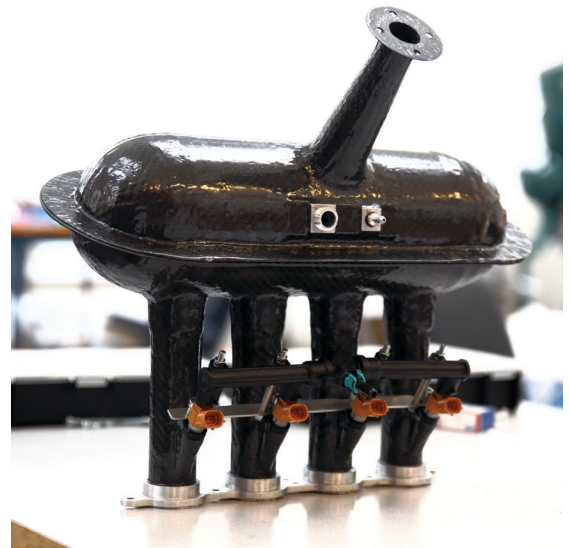
Figure 2: Soluble core eliminated all tooling for this manifold.
