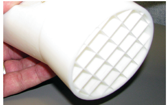
Figure 12: Bottom surface of a soluble mandrel with the cap layers removed (SR-30 white).
