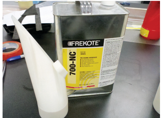
Figure 15: Coat core with a water-based release agent after applying sealant (SR-30 white).
