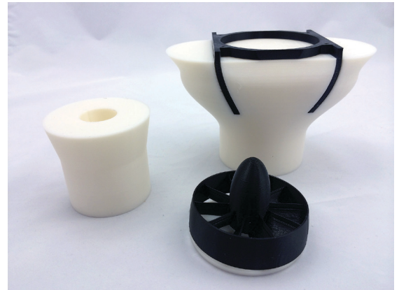
Figure 7: Pockets are left for permanent features to be embedded into the core (ABS-M30 black, and SR-30 white).
