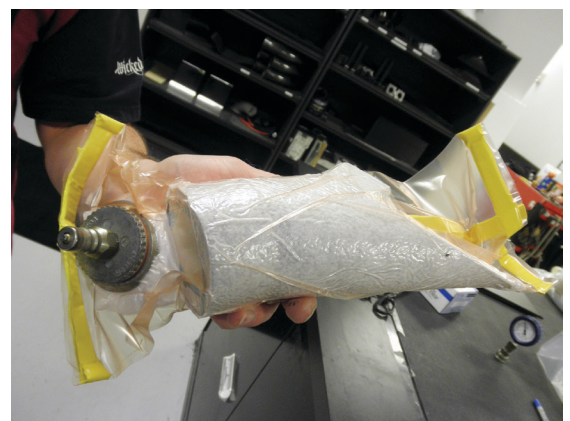
Figure 17: Consolidate composite (vacuum bagging shown).
