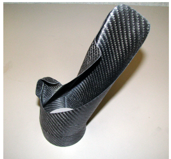
Figure 22: Final product, a composite brake duct, ready for use.
