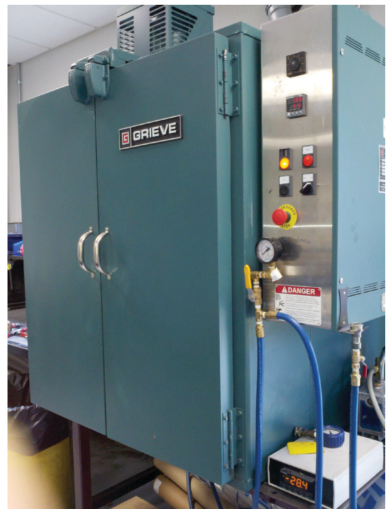
Figure 18: Cure composite parts below 93 °C (200 °F) if using SR-30.
