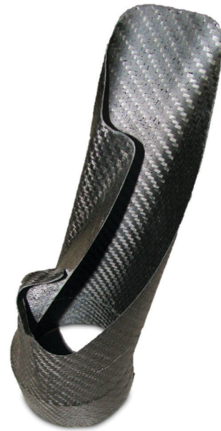
Figure 1: Composite brake duct manufactured from soluble FDM core.
