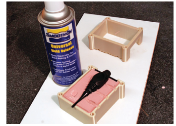
Figure 42: Spray mold release on A-side of mold before pouring B-side.
