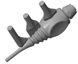
Figure 10: Optionally, add gate and vents to CAD model to construct them as part of the FDM pattern.
