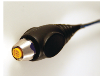
Figure 56: Final cast urethane part – overmolded connector.
