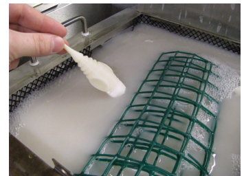
Figure 20: Remove soluble supports in dissolving tank.
