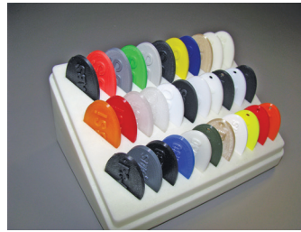
Figure 17: All FDM materials are suitable for RTV patterns.
