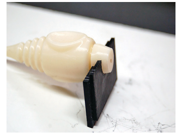
Figure 34: To position the connector that will be overmolded, an endplate (black) is added to the mold.
