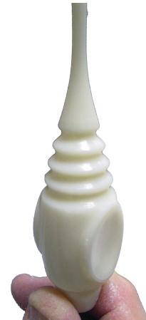
Figure 2: FDM pattern ready for mold making.
