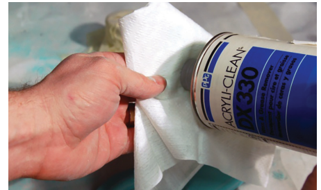
Figure 24: Degrease surfaces between steps to ensure good adhesion of fillers and primers.
