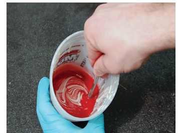
Figure 36: Thoroughly mix the two components of the RTV rubber kit.
