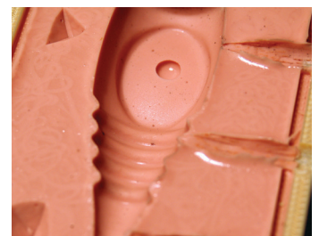
Figure 38: If air bubbles remain in the RTV rubber, they may form voids on the mold's surface.
