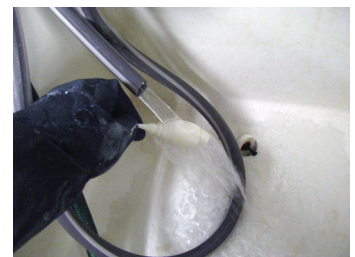
Figure 22: Thoroughly wash pattern to remove dissolving solution.
