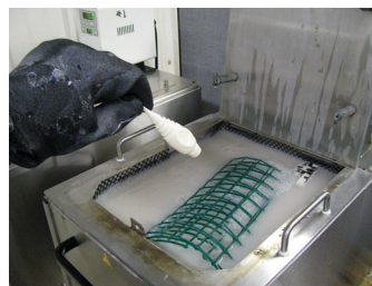
Figure 21: After supports have dissolved, remove pattern from tank.
