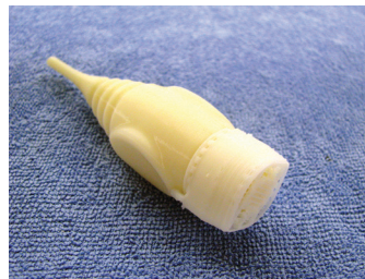
Figure 19: Supports (soluble shown) are removed after FDM construction.
