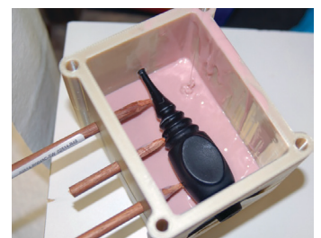
Figure 40: Alternative method — for simple parting lines, eliminate the clay-up step and pour rubber to height of A-side mold box.
