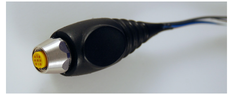
Figure 1: Overmolded connector cast in an RTV mold made from an FDM pattern.
