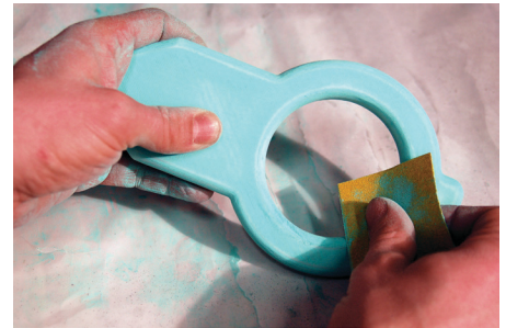
Figure 28: After filler has dried, sand pattern to desired smoothness (alternate part show).
