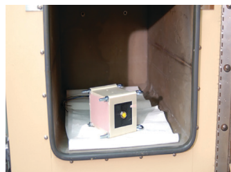
Figure 49: To remove air bubbles, place the mold in a vacuum chamber.
