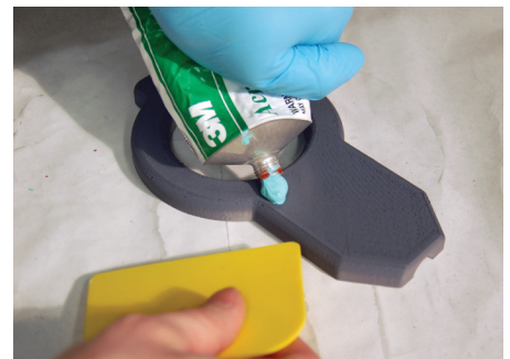
Figure 26: Apply a small amount of filler on pattern (alternate part show).
