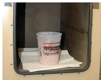
Figure 37: De-air the RTV rubber in a vacuum chamber (shown) or pressure pot.
