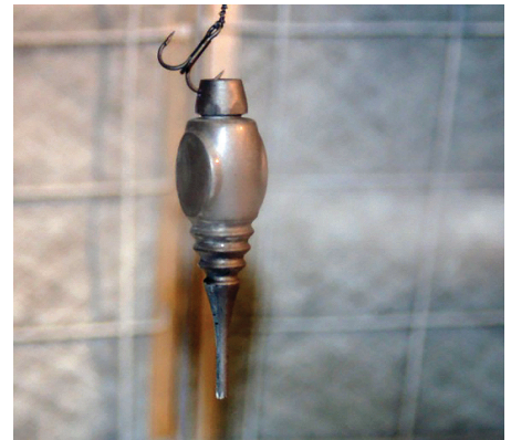
Figure 25: Spray thin coats of primer (optional) onto surface of pattern.
