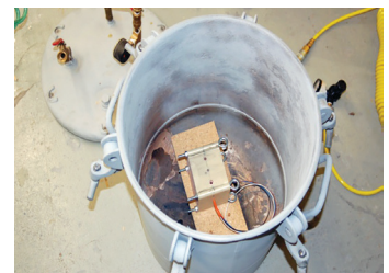
Figure 50: Another option to remove air bubbles from the casting is a pressure chamber.
