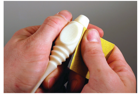
Figure 29: If fillers are not used, sand pattern after support removal.
