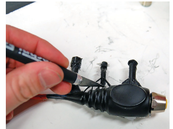
Figure 52: Trim vents and gates from casting.
