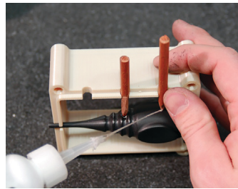
Figure 33: Attach gate and vents (for clarity, parting surface removed and primed pattern used).
