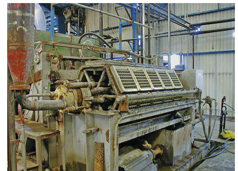
Figure 2: Paper pulp molding machine transfers the mold to the slurry tank and pulls a vacuum to draw pulp against the screen.
