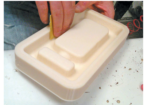
Figure 25: Finish the mold to desired surface smoothness.
