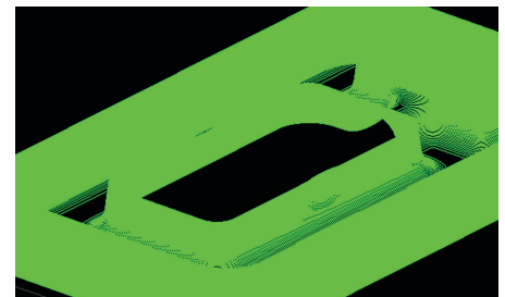
Figure 8: The Internal mesh custom group produces an open, lattice-like structure that preserves vacuum flow.
