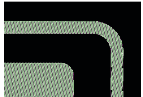
Figure 12: The screen's custom group uses a narrow raster air gap without a perimeter on oddnumbered layers.
