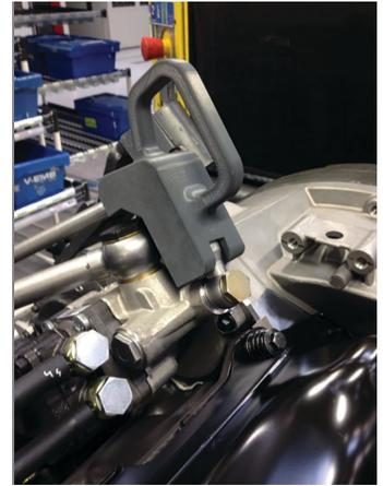
This 3D printed holding fixture (gray) is used to maintain the position of an engine hose during assembly.
