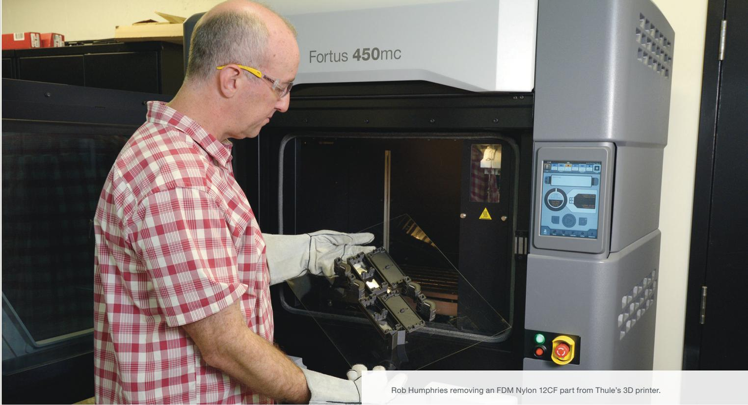
Rob Humphries removing an FDM Nylon 12CF part from Thule's 3D printer.
