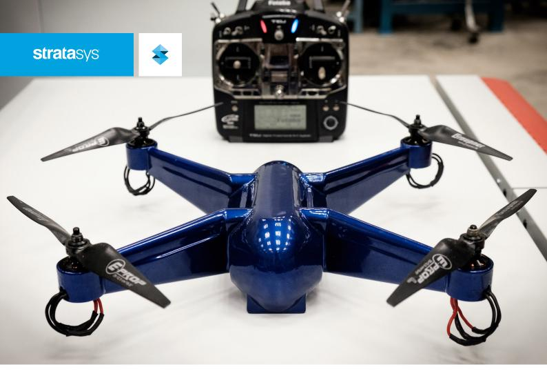
Is it possible to design a drone with commercial off-the-shelf (COTS) electronic hardware that is embedded during the 3D printing process? Is it possible to manufacture a drone that could effectively be ready for flight as soon as it is 3D printed? These questions formed the basis of this project and led to an exploration of hybrid 3D printing and the benefits of embedded hardware.
