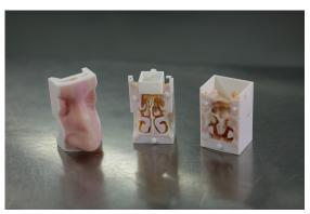
Figure 1: Ear nose throat surgery model in a multi-material jetting 3D printer. Able to achieve resolutions of less than 30 microns, material jetting can replicate fine structures.
