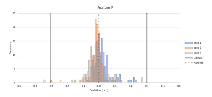
Feature F shows a broad spread, with a few outlier specimens in the extremes of the histogram. The peaks lie within 40µm of each other. It achieves an overall yield of 99.7%, a CPK of 1.6 and the spread is consistent with IT14.
