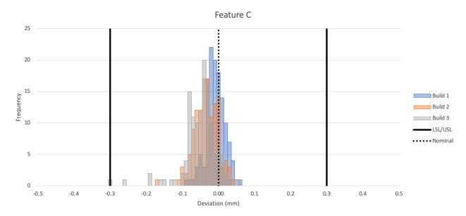
Feature C is very well centred and features minimal outliers. The range between histogram peaks is 42µm and the feature overall achieves a yield of 100%, a CPK of 2.2. The spread is consistent with IT13.
