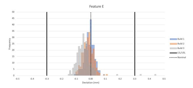
Feature E shows upwards outliers, some of which lie outside the upper spec limit (USL). The consistency between builds is still good, with the range of histogram peaks lying within 39µm of each other. It achieves an overall yield of 99.7%, a CPK of 2.1 and the spread is consistent with IT14.
