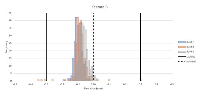
Feature B signifies many of the same behaviors as feature A. This shows tight grouping between builds and a few low outliers that lie outside of the LSL. The histogram peaks all lie within 35µm of each other and the feature overall achieves a yield of 99.5%, a CPK of 2.0 and the spread is consistent with IT14.
