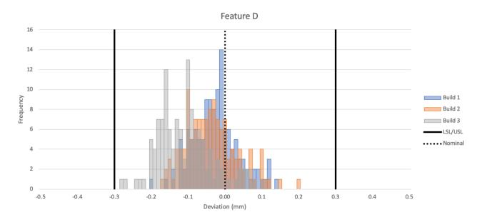
Feature D exhibits a much broader spread than the previous features but is still consistent within builds. It has a range of histogram peaks of 81µm. It also still achieves an overall yield of 100%, a CPK of 1.1 and the spread is consistent with IT15.
