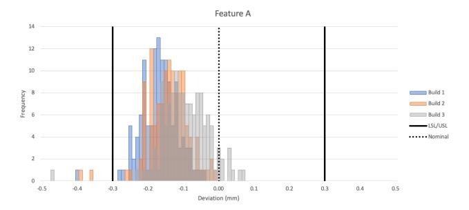
Feature A is mostly in spec but contains some outliers below the lower spec limit (LSL). The individual builds are consistent, with the mean deviation (peak of the histogram) from each build within 75µm. Overall, the feature achieves a 99.0% yield with a CPK of 0.9 and the spread remains consistent with IT15 according to ISO286-1.
