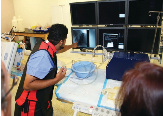
Figure 3: Using 3D printed vascular models in a simulated catheterization lab at the Jacobs Institute.
