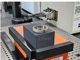
Two examples of 3D printed CMM fixtures used to constrain machined parts.
