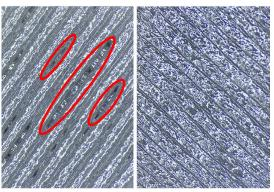
Magnified images of ABS-CF10 with porosity (bead gaps) circled on the left and no gaps after tuning with OpenAM on the right.
