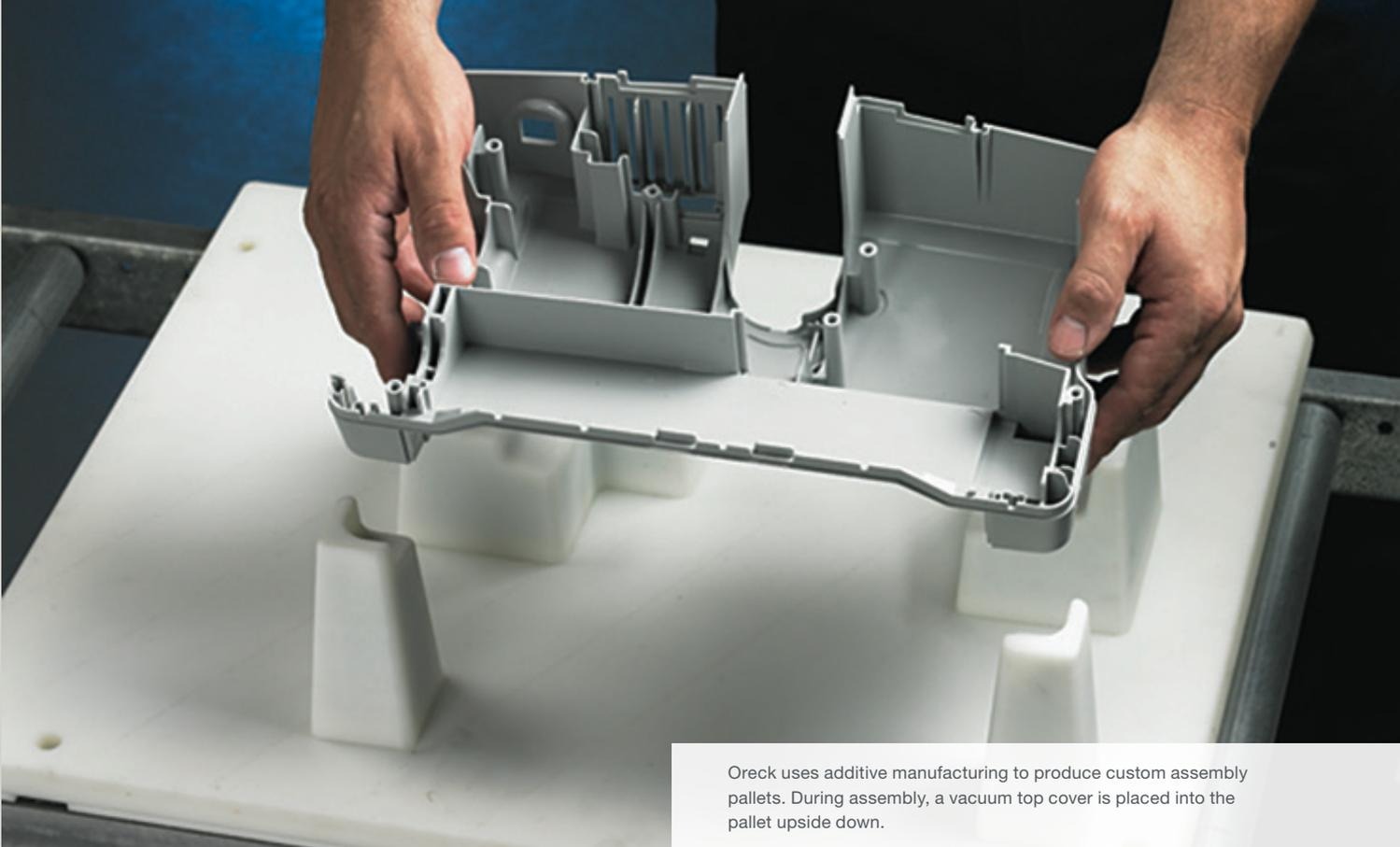
Oreck uses additive manufacturing to produce custom assembly pallets. During assembly, a vacuum top cover is placed into the pallet upside down.
