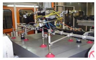
Lifting tool used to move sheet metal blanks.
