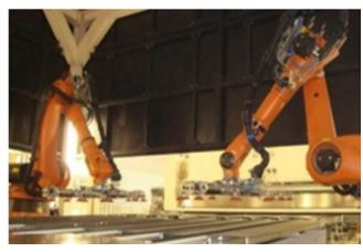
A twin robot assembly used to transfer flat metal blanks.
